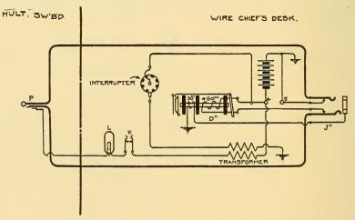
FIG. 470.-TESTING TRUNK TO MULTIPLE BOARD.
