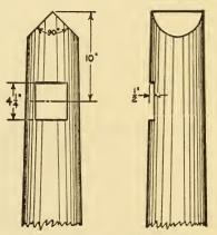
FIG. 543.-ROOFING AND GAINING.
