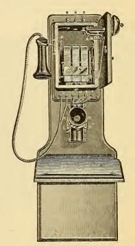
FIG. 115.-COMPLETE WALL TELEPHONE SET.
