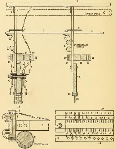
FIG. 454.-DETAILS OF FORD & LENFEST DISTRIBUTING FRAME.
