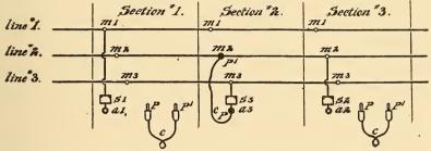
FIG. 201.-ARRANGEMENT OF PARTS IN MULTIPLE SWITCH-BOARD.
