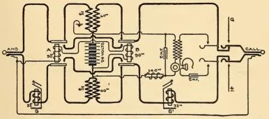
FIG. 306.—WESTERN ELECTRIC CORD CIRCUIT FOR PRIVATE BRANCH EXCHANGE.
