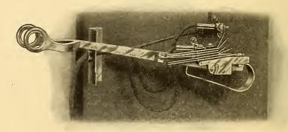
FIG. 263.-DETAIL OF HOOK AND CORD MOUNTING.
