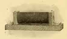
FIG. 59.-INDUCTION COIL WITH TERMINALS ON BASE.
