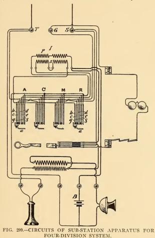
When, however, the subscriber's receiver is hung up current flows from ground at the central office through the battery and the corresponding supervisory relay, thence through one side of the corresponding repeating coil to the ground at the subscriber's instrument. The feature of double supervision is thus secured in accordance with the standard code of signaling.
