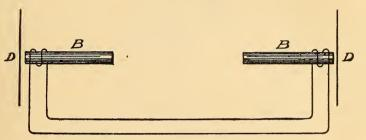
FIG. 9.-BELL MAGNETO TELEPHONE.
