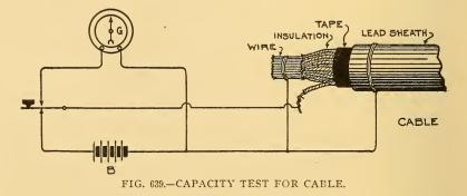
the discharge of the cable produced a deflection twice as great, we would know that the capacity of the cable was  $2 \times \frac{I}{IO} = \frac{I}{5}$  micro-farad.
