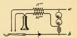
FIG. 256.-WESTERN ELECTRIC SUB-STATION CIRCUIT.
