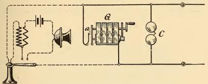
FIG. 111.-BRIDGING CIRCUIT-HOOK DOWN.
