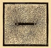
FIG. 2.-LINES OF FORCE OF BAR-MAGNET.
