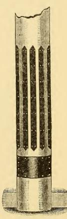
FIG. 536.-POLE STRIPS AND BUTT PLATES.
