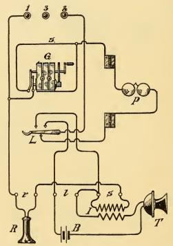
FIG. 113.—CIRCUIT OF COMPLETE SERIES TELEPHONE—COIL IN BASE OF ARM.
