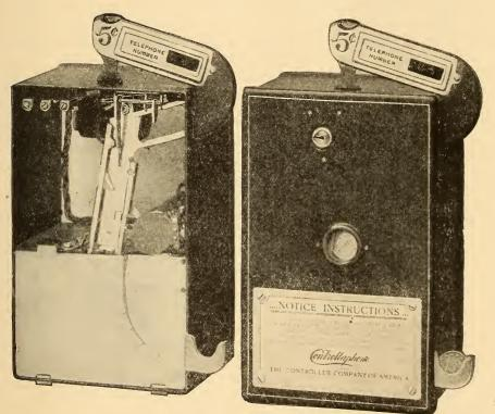
FIG. 345.—STROUD COIN-COLLECTING DEVICE.
