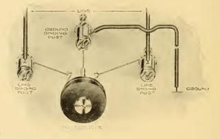
FIG. 439.-CONNECTIONS OF KELLOGG CARBON ARRESTER.
