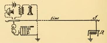
FIG. 159.-CIRCUITS MAGNETO SWITCH-BOARD-SUBSCRIBER CALLING.
