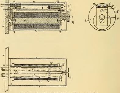
FIG. 389.-WESTERN ELECTRIC CUT-OFF RELAY.
