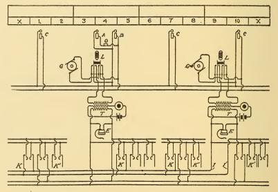
FIG. 222.-TRANSFER AND ORDER-WIRE CIRCUITS.
