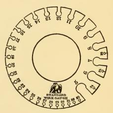
FIG. 534.—CIRCULAR WIRE GAUGE.
