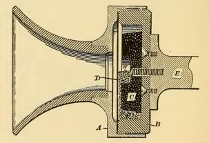
FIG. 54.—WESTERN TELEPHONE CONSTRUCTION COMPANY'S TRANSMITTER.
