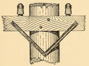
FIG. 542.-METHOD OF ATTACHING BRACES.
