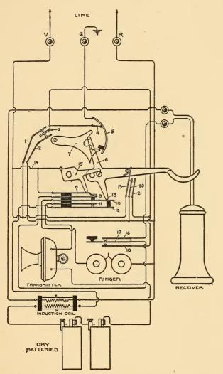
FIG. 511.-CIRCUITS OF SUBSCRIBER'S INSTRUMENT,
