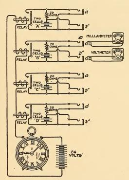
FIG. 74.-METHOD OF TESTING PRIMARY BATTERIES.
