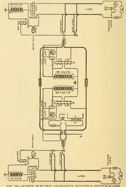
FIG. 277.—NORTH ELECTRIC COMPANY'S MULTIPLE SWITCH-BOARD CIRCUIT. The third contact on the jack is wired through the coil of a cut-off
