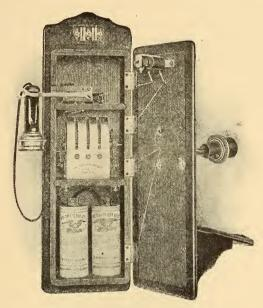
FIG. 120.-DRY-BATTERY WALL SET-OPEN.
