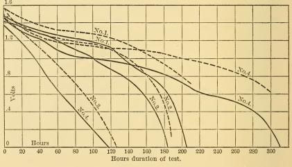
FIG. 76.-CURVES OF BATTERY USING CONSTANT-CURRENT METHOD
