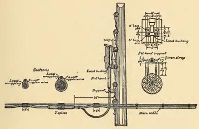
FIG. 610.-DETAILS OF CABLE TERMINAL.
