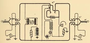
FIG. 205.—CORD CIRCUIT FOR METALLIC CIRCUIT SERIES-ULTIPLE BOARD.
