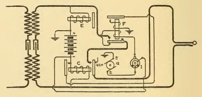
FIG. 291.-KELLOGG AUTOMATIC RINGING CIRCUITS.
