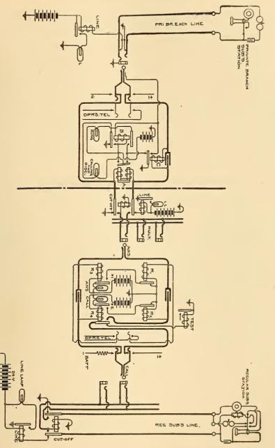
FIG. 314.—CONNECTION BETWEEN PRIVATE-BRANCH AND CITY SUB-SCRIBERS WHEREIN THE PRIVATE-BRANCH SUBSCR'BER CON-TROLS THE SUPERVISORY SIGNAL AT THE MAIN OFFICE.
