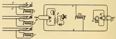
FIG. 167.-SWITCH-BOARD CIRCUIT FOR METALLIC LINES.
