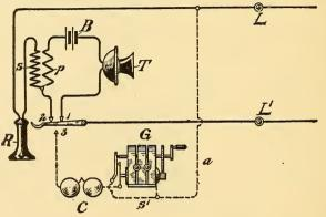
FIG. 108.-SERIES CIRCUIT-HOOK UP.
