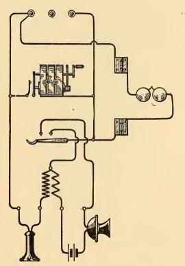
FIG. 118.-BRIDGING CIRCUIT-COIL IN BELL BOX.
