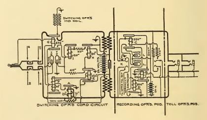
FIG. 353.-WESTERN ELECTRIC TOLL TRUNK LINE, SYSTEM A.
