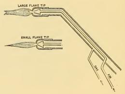
FIG. 417.-BURNER FOR LEAD BURNING.
