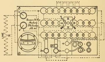
FIG. 628,-PLAN OF PORTABLE TESTING SET.
