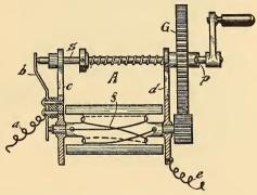
FIG. 87.—AUTOMATIC SHUNT.
