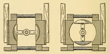
FIG. 84.-DETAILS OF GENERATOR POLE-PIECES.
