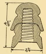
FIG. 545.-DOUBLE-GLASS TRANSPOSITION INSULATOR.
