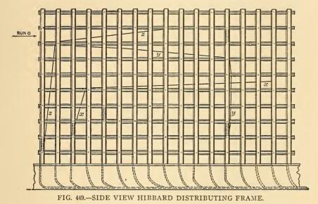
work. As a result of this arrangement channels or horizontal runs are formed for the jumper wires between the vertical and lateral bars, and vertical channels or falls between the sets of intersecting horizontal bars. On the ends of the lateral bars, i, are vertical strips, d and d', of insulating material, upon which are arranged the terminals for the various wires in the cables and the jumpers.
