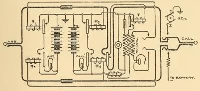
FIG. 270.-COMPLETE KELLOGG CORD CIRCUIT.
