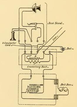
FIG. 129.-BRIDGING DESK SET CIRCUIT-COIL ON RACK.
