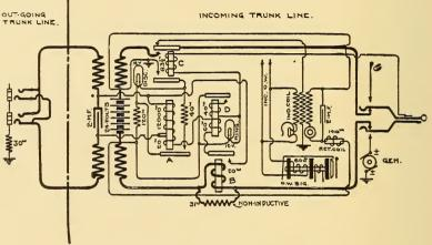
FIG. 286.-WESTERN ELECTRIC TRUNK CIRCUIT.
