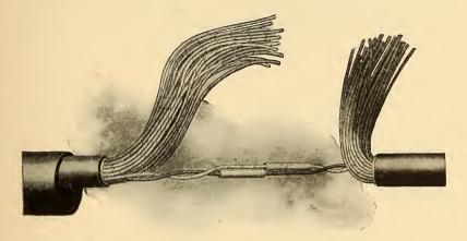
FIG. 601.-CABLE SPLICING.
