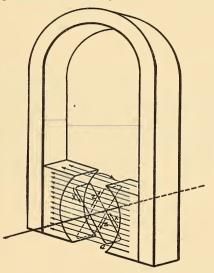
FIG. 77.-FIELD OF FORCE IN MAGNETO GENERATOR.
