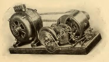
FIG. 405.—RINGING MACHINE WITH BUSY-BACK ATTACHMENT BELTED TO ALTERNATING-CURRENT MOTOR.
