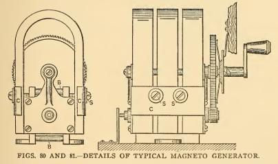
stick to one pole or the other of the magnets. The two coils are oppositely wound, and when a current passes through them it strengthens the magnetism of one pole and weakens that of the other. The next instant the current reverses, and the strong pole
