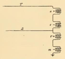
FIG. 297.—SIMPLIFIED LINE SIGNALING CIRCUIT.
