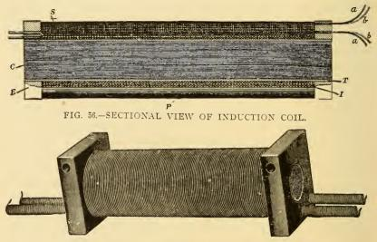
FIG. 57.-PERSPECTIVE VIEW OF INDUCTION COIL.
