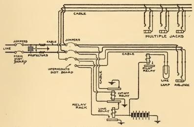
FIG. 458.—DIAGRAM OF CONNECTIONS THROUGH INTERMEDIATE DISTRIBUTING FRAME—WESTERN ELECTRIC SYSTEM.
