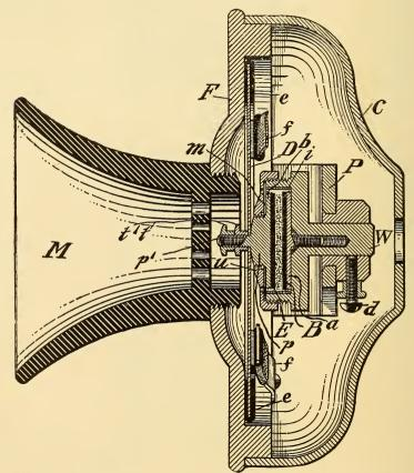
FIG. 45.—SECTIONAL VIEW OF SOLID-BACK TRANSMITTER.
