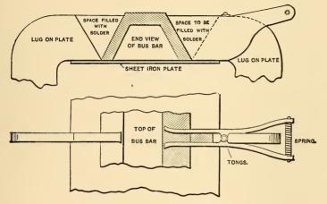
FIG. 420.-METHOD OF BURNING LUGS TO BUS-BARS.
