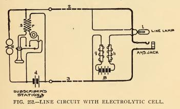
of the scheme already mentioned of placing a secondary battery at the sub-station charged from the central office over the line circuit.
