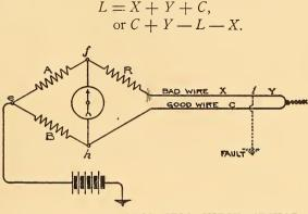
FIG. 642 .- VARLEY LOOP TEST-CHECK METHOD.
