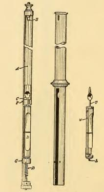
FIG. 631.-SUSPENSION OF D'ARSONVAL GALVANOMETER.
