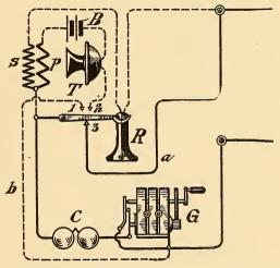
FIG. 109.-SERIES SHUNTING CIRCUIT-HOOK DOWN.
