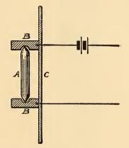
FIG. 19.-HUGHES' CARBON MICROPHONE.
