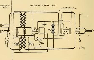
FIG. 289.-KELLOGG TRUNK CIRCUIT.
