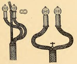
FIG. 39.-SUPPORTING LOOP AND HOOK FOR RECEIVER CORD.
