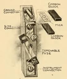
FIG. 429.—COMBINED FUSE AND CARBON ARRESTER SINGLE CONDUCTOR.
