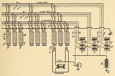
FIG. 207.—SIMPLIFIED DIAGRAM OF BRANCH TERMINAL MULTIPLE BOARD.
