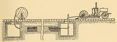
FIG. 620.-DRAWING IN BY STEAM POWER.
