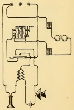
FIG. 117.-SERIES CIRCUIT-COIL IN BELL BOX.
