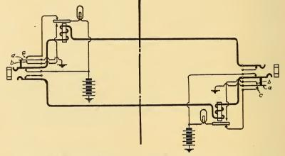
FIG. 312.—TWO-WAY TRUNK CIRCUIT BETWEEN TWO PRIVATE-BRANCH SWITCH-BOARDS—CHICAGO TELEPHONE COMPANY.
