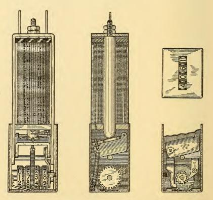
FIG. 352.-WESTERN ELECTRIC CONNECTION METER.
