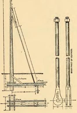
FIG. 563.—DETAILS OF ANCHOR POLE.
