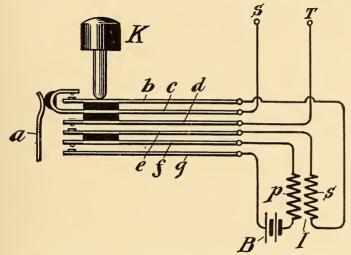
FIG. 300.-DETAIL OF SUBSCRIBER'S SIGNALING APPARATUS.
