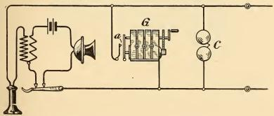
FIG. 112.-BRIDGING CIRCUIT-HOOK UP.
