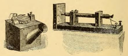
FIGS. 6 AND 7.-REIS' TELEPHONE TRANSMITTER AND RECEIVER.
