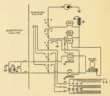
FIG. 515 .- FIRST SELECTOR DURING TIME OF ACTION.
