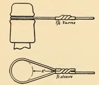
FIG. 585.-DEAD-ENDING WITH MCINTYRE SLEEVE.
