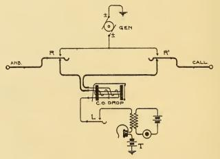
FIG. 203.-CORD CIRCUIT FOR SERIES-MULTIPLE BOARD.
