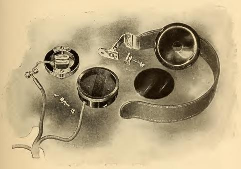
FIG. 34.-PARTS OF WATCH-CASE RECEIVER.
