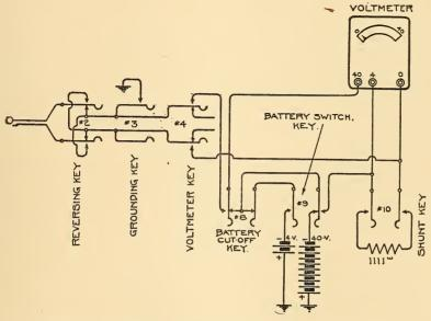
FIG. 473.-VOLTMETER CONNECTIONS OF TESTING CIRCUIT.
