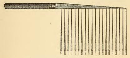
FIG. 476.-METHOD OF FANNING OUT CABLES.
