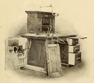
FIG. 317.-PRIVATE-BRANCH EXCHANGE SWITCH-BOARD.
