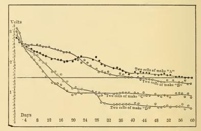
FIG. 75.-CURVES OF BATTERY TESTS, CONSTANT-RESISTANCE METHOD.
