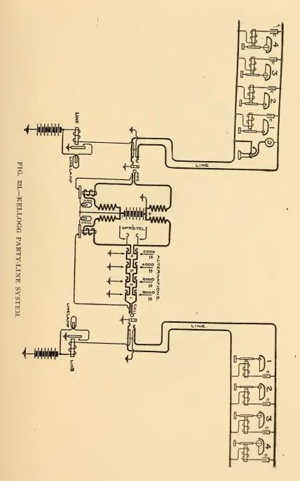
scriber's station, besides the usual talking apparatus, the bell magnet, with its tuned reed and bell tapper, is bridged across the line in series with a condenser, *C*. Currents of 2000, 4000, 6000 and 8000 alternations per minute are used, these currents being sup-
