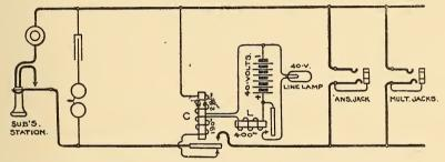
FIG. 271.—STROMBERG-CARLSON TWO-WIRE MULTIPLE SWITCH-BOARD LINE CIRCUIT.
