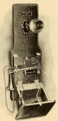
FIG. 262.-COMMON BATTERY WALL SET-OPEN.
