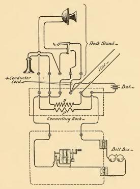
FIG. 128.-SERIES DESK SET CIRCUIT-COIL ON RACK.
