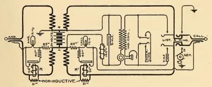
FIG. 265.-WESTERN ELECTRIC MULTIPLE SWITCH-BOARD CORD CIRCUIT.
