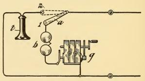
FIG. 106.-HAND-SWITCH CIRCUIT.
