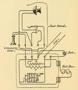
FIG. 127.-BRIDGING DESK SET CIRCUIT-COIL IN BELL BOX.
