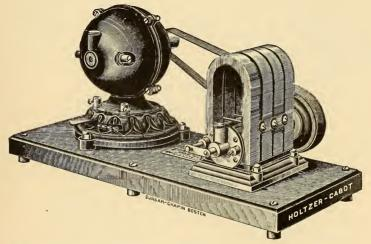
FIG. 402.-MAGNETO GENERATOR BELTED TO DIRECT-CURRENT MOTOR.
