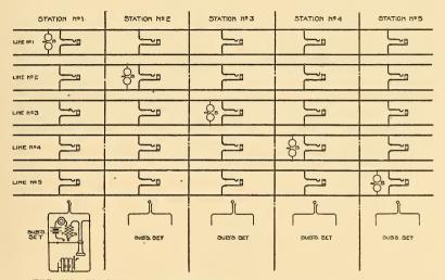
FIG. 527.—MAGNETO INTERCOMMUNICATING SYSTEM, METALLIC CIRCUITS.
