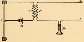
FIG. 21.-TRANSMITTER WITH INDUCTION COIL.
