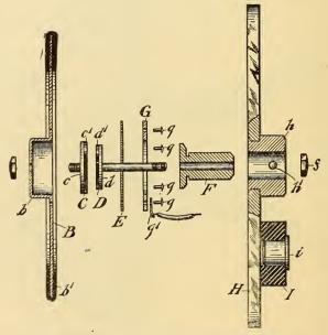
FIG. 48.-DETAILS OF KELLOGG TRANSMITER.
