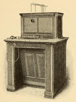
FIG. 253.-COMMON-BATTERY SWITCH-BOARD FOR SMALL EXCHANGES.
