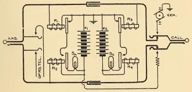
FIG. 269.—KELLOGG MULTIPLE SWITCH-BOARD CORD CIRCUIT SIMPLIFIED.
