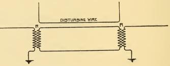
FIG. 150.-ELIMINATING LOCAL INDUCTION.
