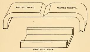
FIG. 418.-METHOD OF BURNING SMALL TERMINALS.
