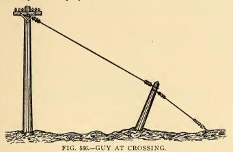
top and bottom arm. To guy from the top of the pole only, as is frequently done, causes the latter to bow toward the center of the
