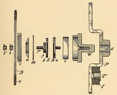
FIG. 46.-DETAILS OF SOLID-BACK TRANSMITTER.
