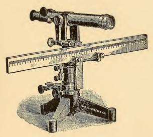
FIG. 632.—SCALE AND TELESCOPE.
