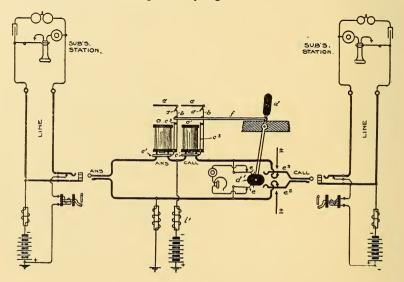
FIG. 249.—SCRIBNER COMMON-BATTERY SYSTEM.
