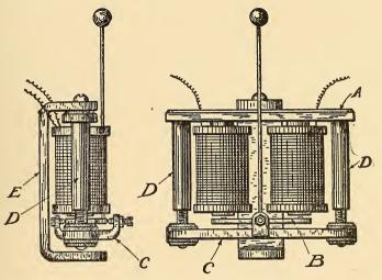
FIG. 83.-TYPICAL MAGNETO BELL.
