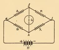
FIG. 626.-DIAGRAM OF WHEATSTONE BRIDGE.
