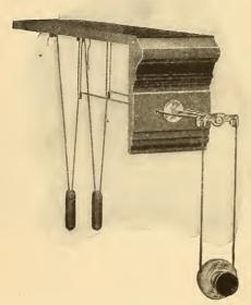
FIG. 384.—OPERATOR'S TRANSMITTER MOUNTING FOR MULTIPLE BOARDS.
