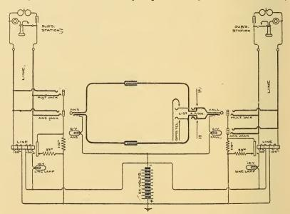
FIG. 274.-CIRCUITS OF STERLING MULTIPLE SWITCH-BOARD.
