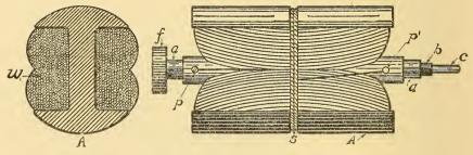
FIG. 78.—ARMATURE OF MAGNETO GENERATOR.
