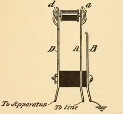
FIG. 426.-HEAT COIL AND HOLDER.
