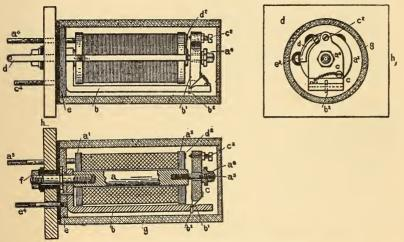
FIG. 388.—WESTERN ELECTRIC LINE RELAY.
