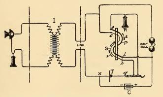
FIG. 257.-WESTERN ELECTRIC SUB-STATION CIRCUIT.
