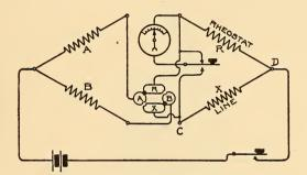
FIG. 629.-CIRCUITS OF PORTABLE TESTING SET.
