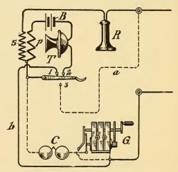
FIG. 110.—SERIES SHUNTING CIRCUIT—HOOK UP.
