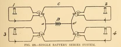
that it was possible to supply all of the cord circuits from a single battery by connecting them in the manner shown in Fig. 228. This involves the bunching together of one side of each of the cord circuits, the battery supplying current in multiple to the various pairs of lines in use at one time. This figure shows four stations, I, 2, 3 and 4, connected in pairs by two cord circuits and pairs of plugs.
