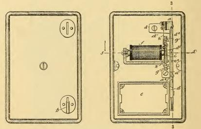
FIG. 341-SCRIBNER COIN-COLLECTING DEVICE.
