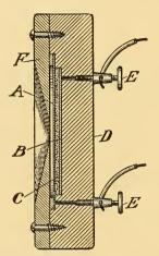
FIG. 20.-HUNNING'S GRANULAR CARBON TRANSMITTER.
