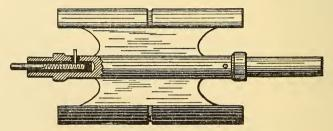
FIG. 82.-ARMATURE CORE OF TYPICAL GENERATOR.
