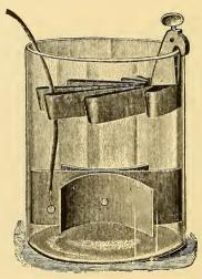
FIG. 71.-THE GRAVITY CELL.
