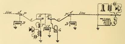
FIG. 161.-CIRCUITS MAGNETO SWITCH-BOARD-CALLING SUBSCRIBER.
