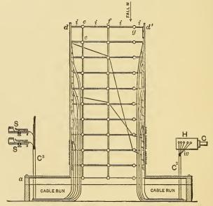
FIG. 448.-END VIEW HIBBARD DISTRIBUTING FRAME.
