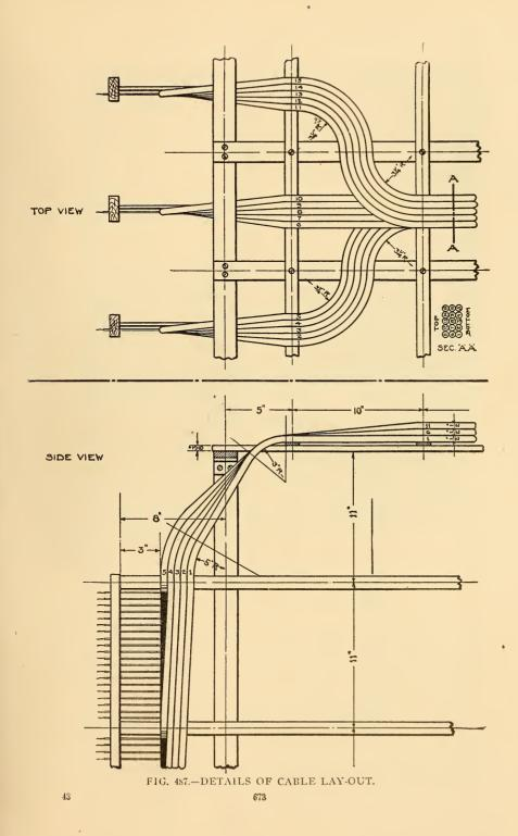
work is done in designing the wiring, why practically all of the cables, both long and short, should not be prepared, cut to length, formed, and in some cases soldered to their terminals in the factory rather than doing it at the installation. To do this, however, requires the utmost nicety in the laying out of the various details of the plant.
