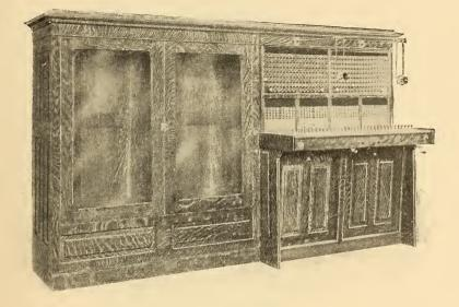
FIG. 196.—TWO-POSITION STROMBERG-CARLSON BOARD WITH TERMINAL CABINET.
