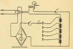
FIG. 467.-TESTING PLUG CIRCUIT.
