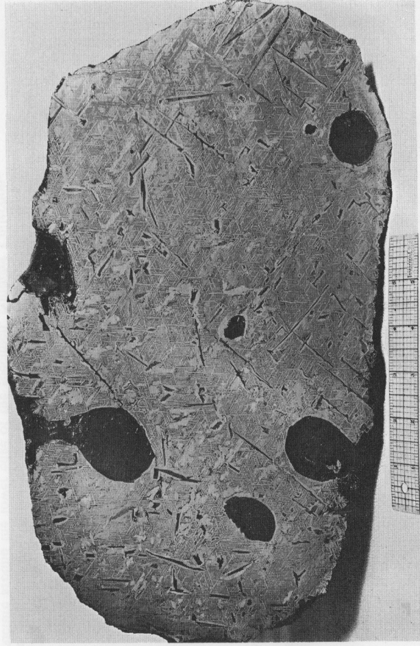
Fig. 19. Polished and etched section of the Bear Creek, Colorado, meteorite exhibiting fine octahedral structure. The bar-like inclusions which interrupt the Widmanstätten pattern are schreibersite. The rounded nodules are troilite. Nininger Collection.
