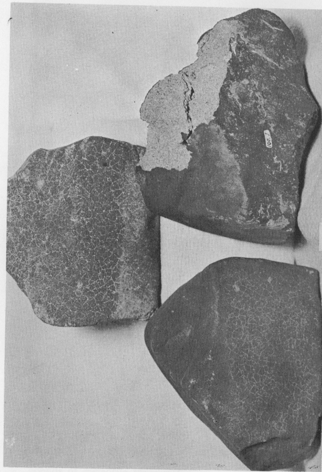
Fig. 4. A group of stony meteorites which fell near Richardson, North Dakota, on June 30, 1918. The stony interior is gray with the black fusion crust showing many minute contraction cracks. The specimen on the lower right has uncharred straw fibers still clinging to it. (Bar equals one inch.) Nininger Collection.
