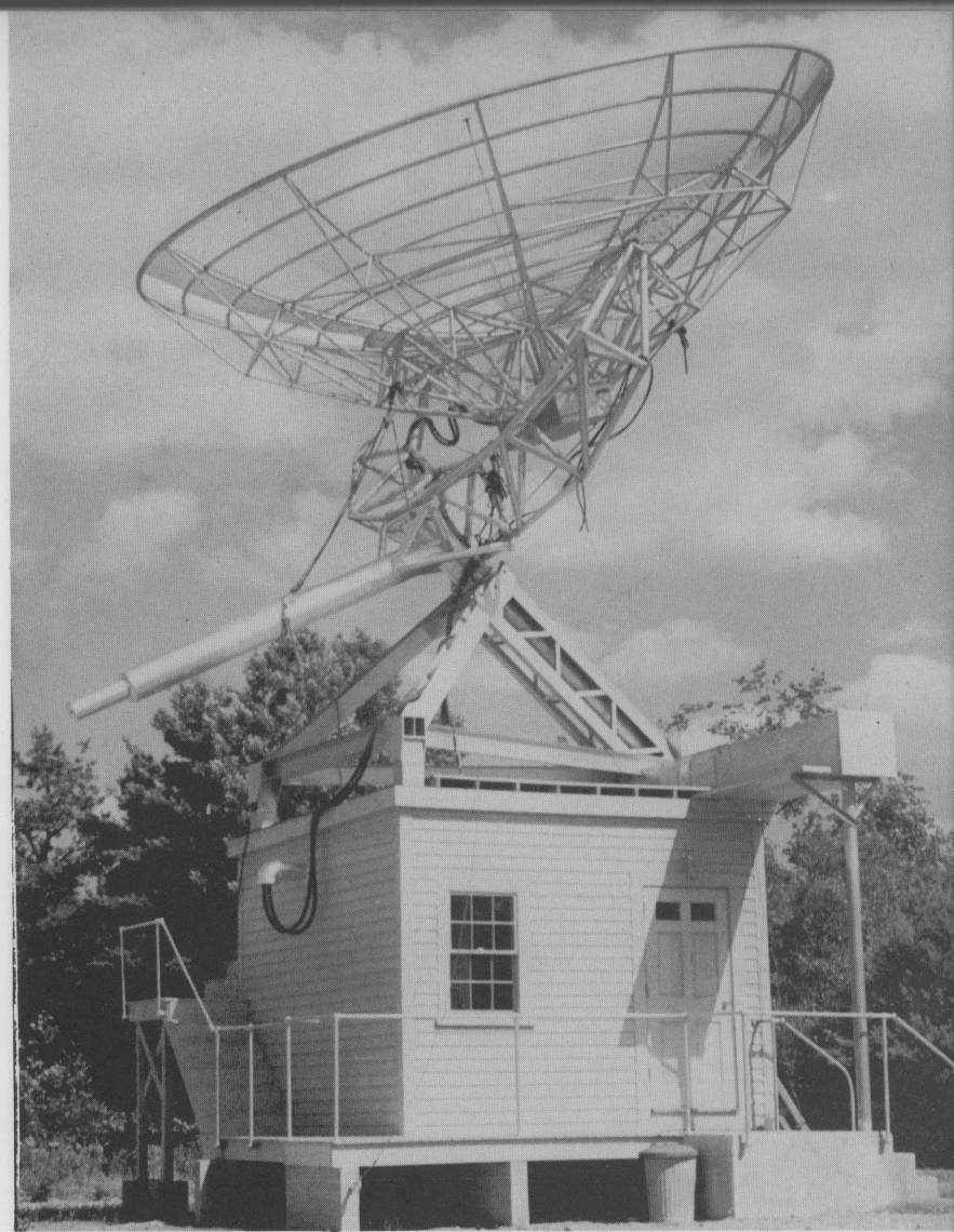
Fig. 48. 25 foot Radio Telescope at Harvard Observatory. Can "see through" dust clouds, using the same principles as radar (see page 130).
