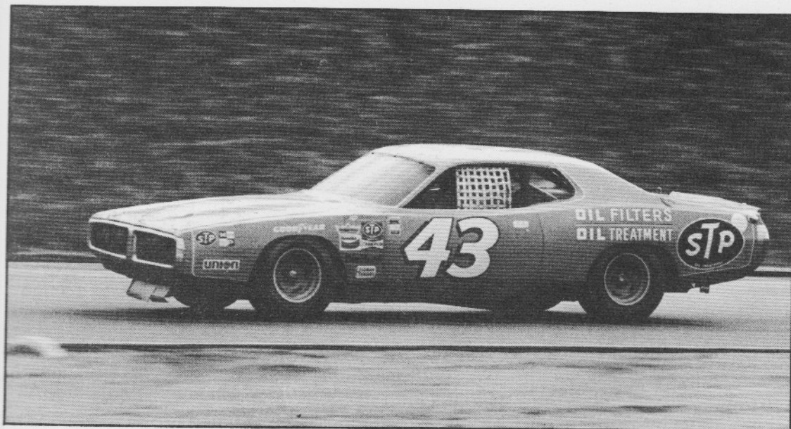
Richard Petty's Dodge Charger was one of the more aerodynamic cars ever to road race. Despite the smooth contours, the "air-fol" shape that tends to produce undesirable lift at high speed is still very evident. Note the front and rear spoilers added to resist this upward lift.
