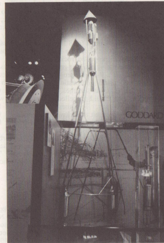
The original Hoopskirt rocket at the National Air and Space Museum. The upper hoop is missing from the rocket, reconstructed from wreckage. (photo by author)
