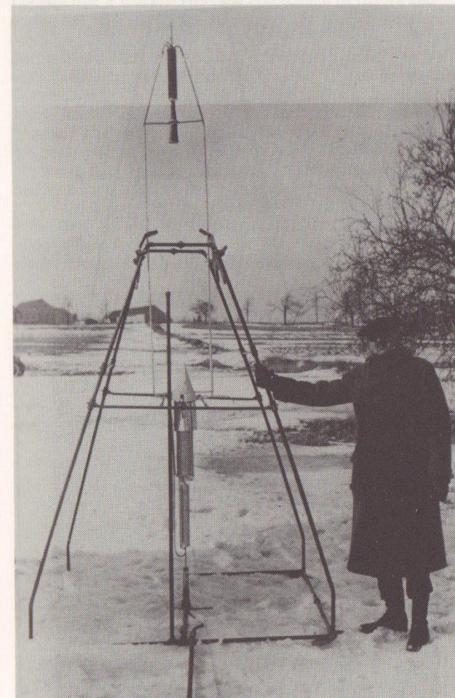
Above: The first liquid-propelled rocket to take flight, shown here on March 16, 1926. The guides at the top of the launcher differ slightly from those in a more famous photo taken a few days earlier. (courtesy of Clark University Goddard Library Archives)
