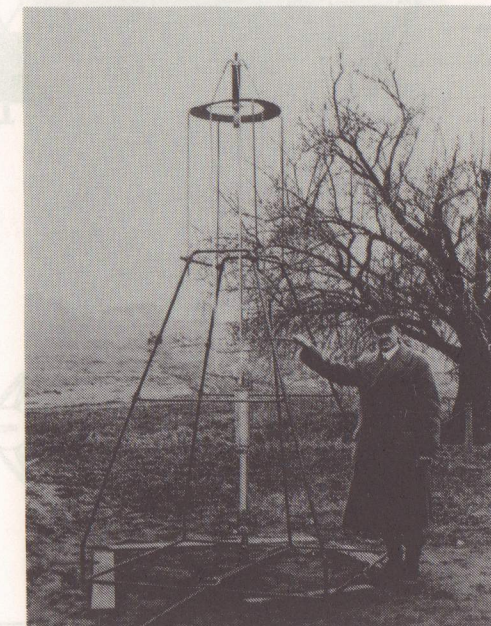
Above: The first liquid-propelled rocket to take flight, shown here on March 16, 1926. The guides at the top of the launcher differ slightly from those in a more famous photo taken a few days earlier. (courtesy of Clark University Goddard Library Archives)
