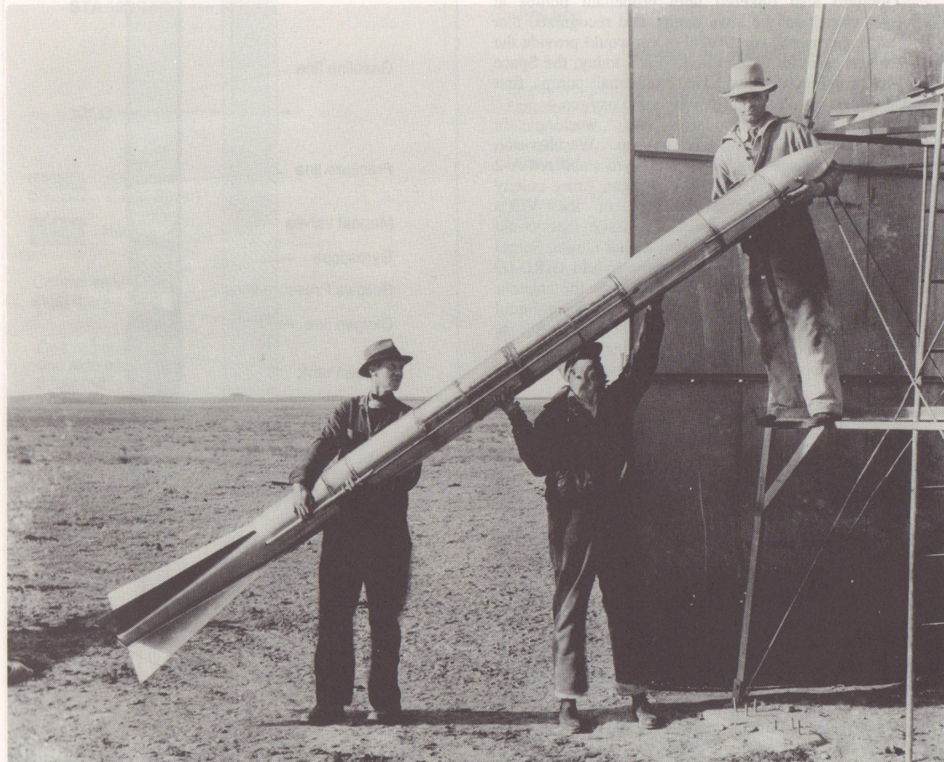
The first A-series rocket flight was test A-3, a simplified model without a guidance system. Throughout the A-series, Goddard repaired and re-used rockets as much as possible—whether the first A-series tests were three flights of one rocket or three rockets of one type is a matter of semantics. (courtesy of Clark University Goddard Library Archives)
