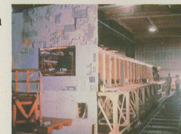
ABOVE: The Death Star model surface-to-tunnel set up. The Vista Cruiser Camera will first move along the surface (vertically mounted) and then enter the opening, trucking down the tunnel (parallel to the camera track).
