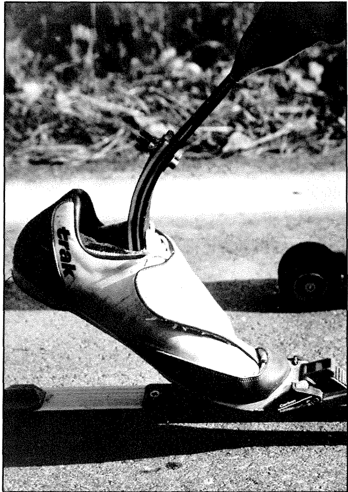
AMERICAN ACADEMY OF ORTHOTISTS AND PROSTHETISTS The Flex-Foot is shown positioned on the roller-ski and in the kicking motion of cross-country skiing.
