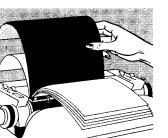
1. Assemble paper for insertion (original on top; second sheets beneath). Turn the "pack" so original faces away from you and the top edge faces down.
